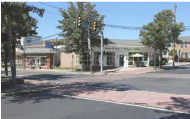
Decorative brick crosswalks at the intersection of Main Street and Walnut Street draw greater attention to pedestrian movements.
