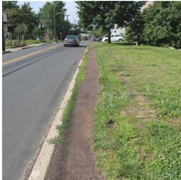
Well-worn pathways called “desire lines” indicate areas that could benefit from a formal sidewalk.
